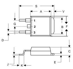
PIN 1. BASE PIN 2. COLLECTOR PIN 3. EMITTER
