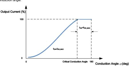
Figure.2 Dimming Curve
