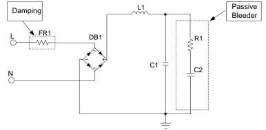
Figure.3 LED Driver Schematic with Passive Bleeder
