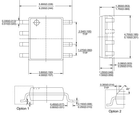
Note: Eject hole, oriented hole and mold mark is optional.
