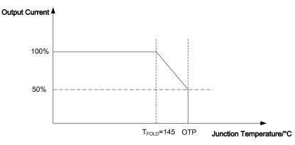
Figure. 1 Thermal Foldback Waveform
