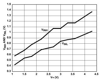
FIGURE 16. DIGITAL SWITCHING POINT vs SUPPLY VOLTAGE
