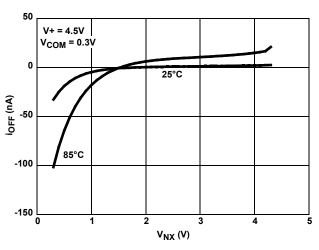
FIGURE 22. OFF LEAKAGE vs SWITCH VOLTAGE
