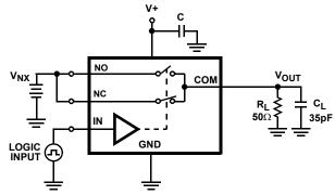
C<sub>L</sub> includes fixture and stray capacitance.
