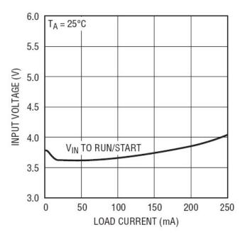
Figure 2. DC1382 Minimum Input Voltage
