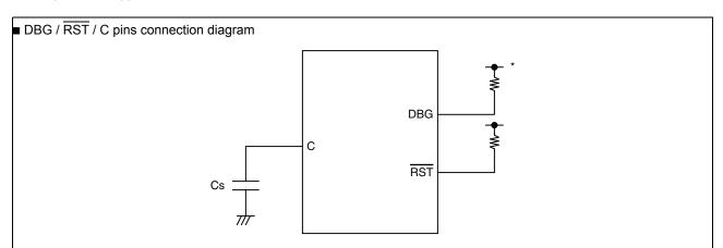
\*: Connect the DBG pin to an external pull-up resistor of 2 kΩ or above. After power-on, ensure that the DBG pin does not stay at "L" level until the reset output is released. The DBG pin becomes a communication pin in debug mode. Since the actual pull-up resistance depends on the tool used and the interconnection length, refer to the tool document when selecting a pull-up resistor.
