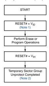
Figure 7.2 Temporary Sector Group Unprotect Operation
