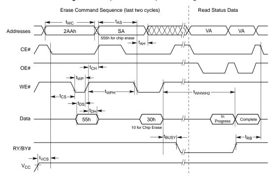
Figure 18.6 Chip/Sector Erase Operation Timings
