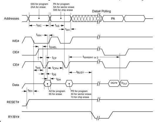
Figure 18.12 Alternate CE# Controlled Write Operation Timings
