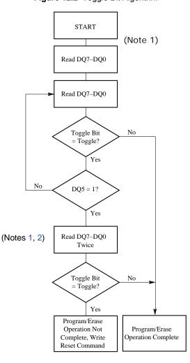
Figure 12.2 Toggle Bit Algorithm
