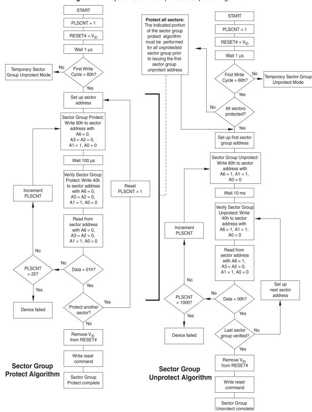
Figure 7.1 In-System Sector Group Protect/Unprotect Algorithms
