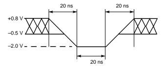
Figure 14.2 Maximum Positive Overshoot Waveform
